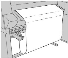
**11** On the Media Take-up Unit, press down the take-up switch to take up about two complete roll turns of media.
